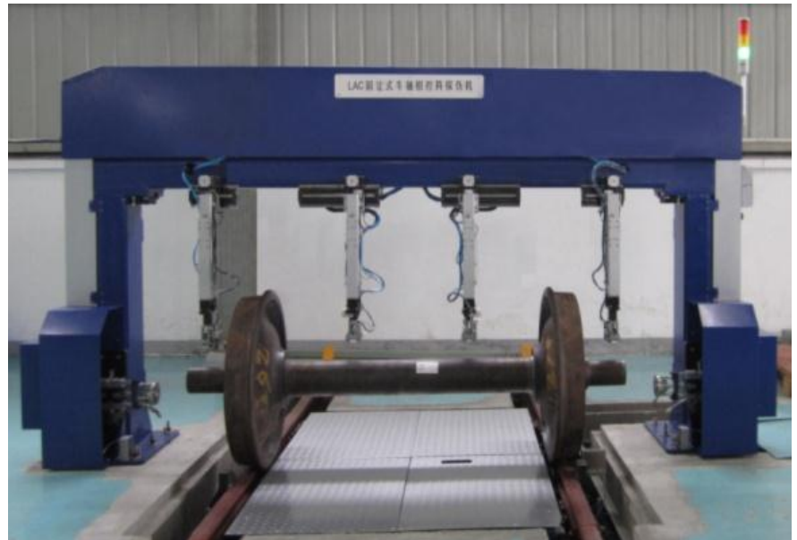
System for axle inspection
